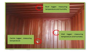
Figure 9: Configuration of logger placement in the container
